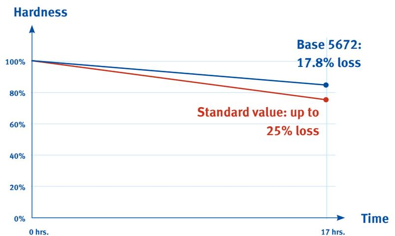
**Static ageing test: EUCABASE® with a lower loss of hardness compared to conventional foams**
