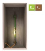
EN 60332-1-2 - vertical flame propagation – describes the testing method for  $\rm E_{Ca}$  and  $\rm F_{Ca}$  classification and is mandatory as well for all higher classifications,  $\rm D_{Ca}$  up to  $\rm B2_{Ca}$
