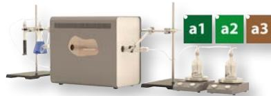
EN 60754-2 describes the testing method for additional criteria with regards to **acidity**  $a1 - a3$  by measuring pH & conductivity
