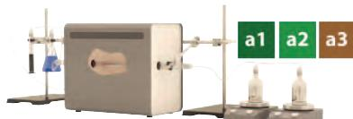
**EN 60754-2** describes the testing method for additional criteria with regards to **acidity** a1 – a3 **by measuring pH & conductivity**
