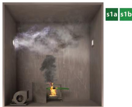
**EN 61034** describes the testing method for additional criteria with regards to **smoke** s1a and s1b (optional)
