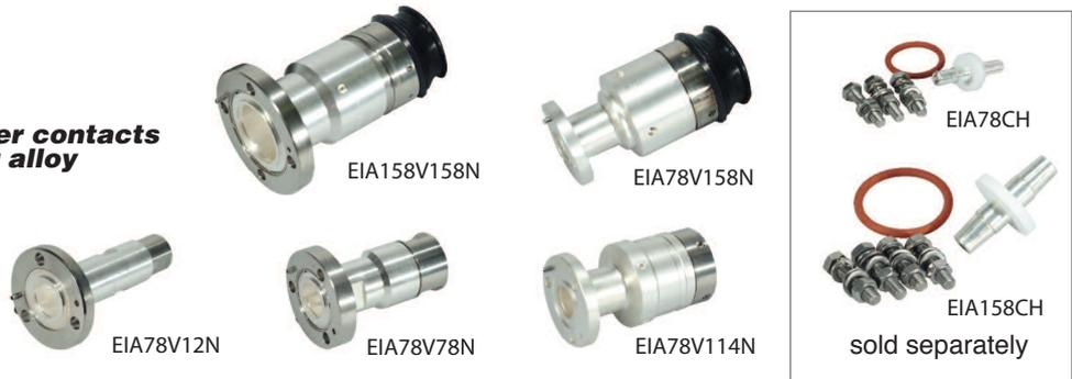
Connectors with EIA 7/8" or EIA 1-5/8" flanges for 1/2", 7/8", 1-1/4" and 1-5/8" cables. The connectors are easy to install. Contact surfaces are silver plated to obtain a low contact resistance and very low intermodulation. Watertightness is achieved by using high-quality o-rings. The straight coupling adapter (with O-ring and bolts), for mating two EIA interfaces together, is sold separately.
